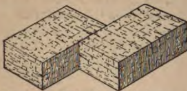
FIG. 57. — A fault of lateral displacement.
